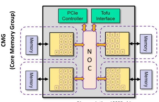
Diagram is the "1000" chip. We have "700" chip, i.e. no assistant cores and no Tofu interface
