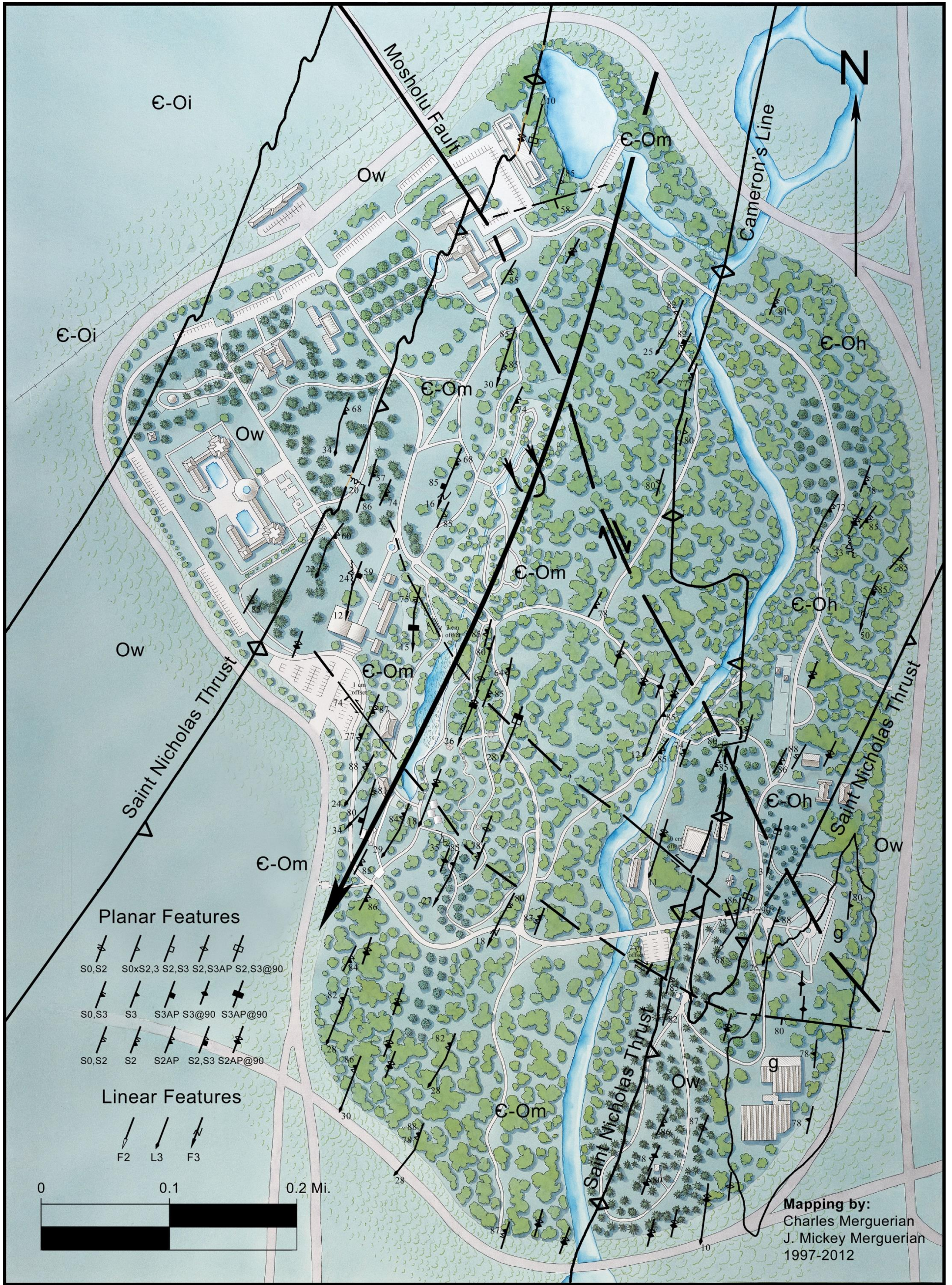
Plate 2 – Uncolored preliminary geological map of the New York Botanical Garden showing the ductile faults (Cameron’s Line and Saint Nicholas thrust) and brittle faults including the Mosholu fault, associated splays and other mapped brittle faults. Units - ε-Oi = Inwood Marble, Ow = Walloomsac Formation, ε-Om = Manhattan Formation, ε-Oh = Hartland Formation, g = foliated late syn-tectonic granitoid. Foliation and bedding (planar features) and fold axes and lineations (linear features) symbols explained in legend with dip and plunge values plotted. Map scale synformal NW-vergent F 3 axial surface trace shown. See Plate 3 for sample and stop locations plotted on park trail map. Basemap courtesy NYBG.
