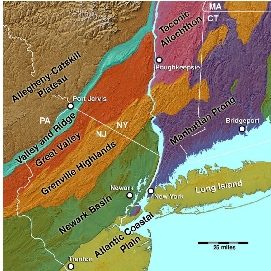
Figure 2 – Physiographic diagram showing the major geological provinces in southern New York, northern New Jersey, and adjoining states. The NYBG is within the Manhattan Prong. (From Bennington and Merguerian, 2007.)
