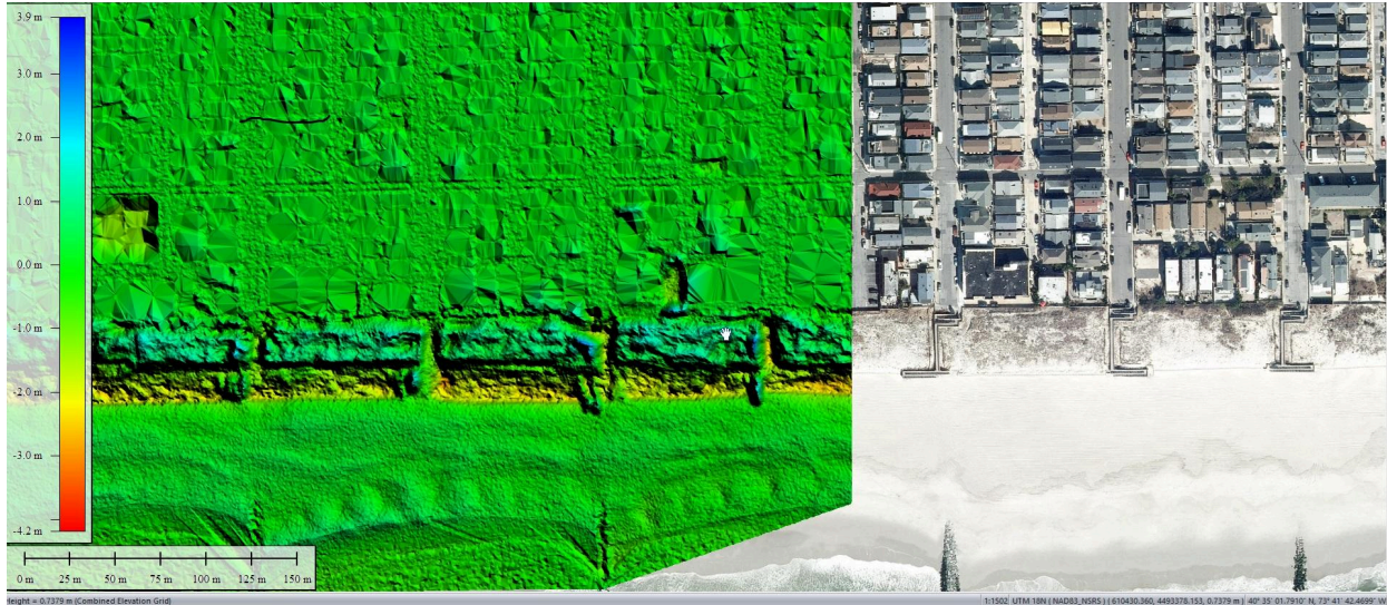
Figure 2: Digital Elevation Model (DEM-DIF) of the difference in meters above sea level in 2011 to 2014 using LiDAR data of a portion of Long Beach coast on the south side of the island. Half of the model was replaced with satellite imagery of the same area for better comparison. The areas in red represent significant land change caused by erosion; the loss in land was around 3.1 meters. The blue represents deposition and was up to 3 meters. The impact of dunes on coastal erosion can also be observed. The areas before the dunes have lost a little more than 2 meters worth of elevation, but the dunes gained 2-3 meters of height where the vegetation is.
