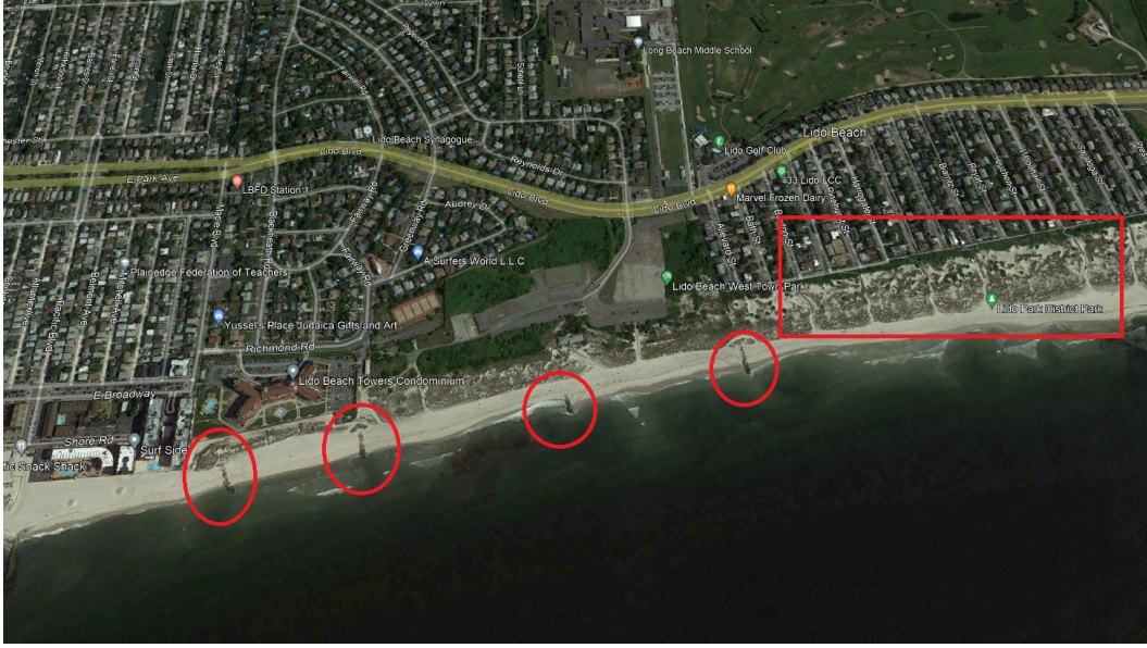
Figure 6: Satellite image of Long Beach taken at 4938ft, June 2010. The image, taken from Google Earth, marks previous vegetation and the jettie system present before significant erosion.
