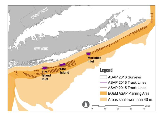
Figure 1. New seismic and core data were collected during 2015 and 2016 from offshore New York as part of the BOEM Atlantic Sand Assessment Project (ASAP). Regional, reconnaissance-level lines were run in Federal waters at a distance of 3 to 8 nautical miles offshore in 2015 while design-level surveys were conducted in three areas in 2016. In addition to seismic profiles and sediment samples, the surveys also collected side-scan sonar, bathymetric and magnetometer data.
