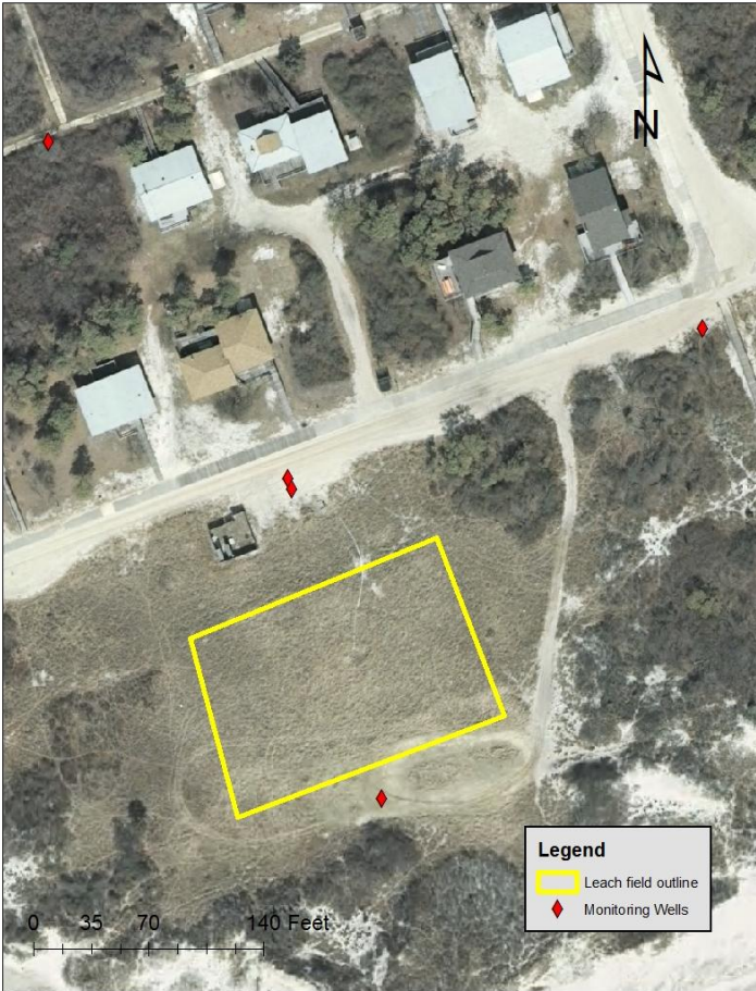
Figure 1 Watch Hill National Seashore field area. Five monitoring wells were sampled in this study. Leach field area is outlined to show proximity to monitoring wells.
