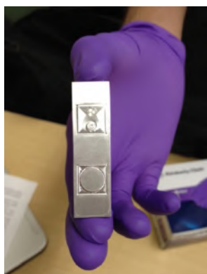
Figure 1: The aluminum mold used to create our backflow inhibitors.
