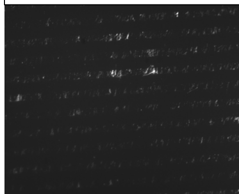
Figure 2. DNA was systematically cut along the lines of the stamp, even in extremely dense conditions.
