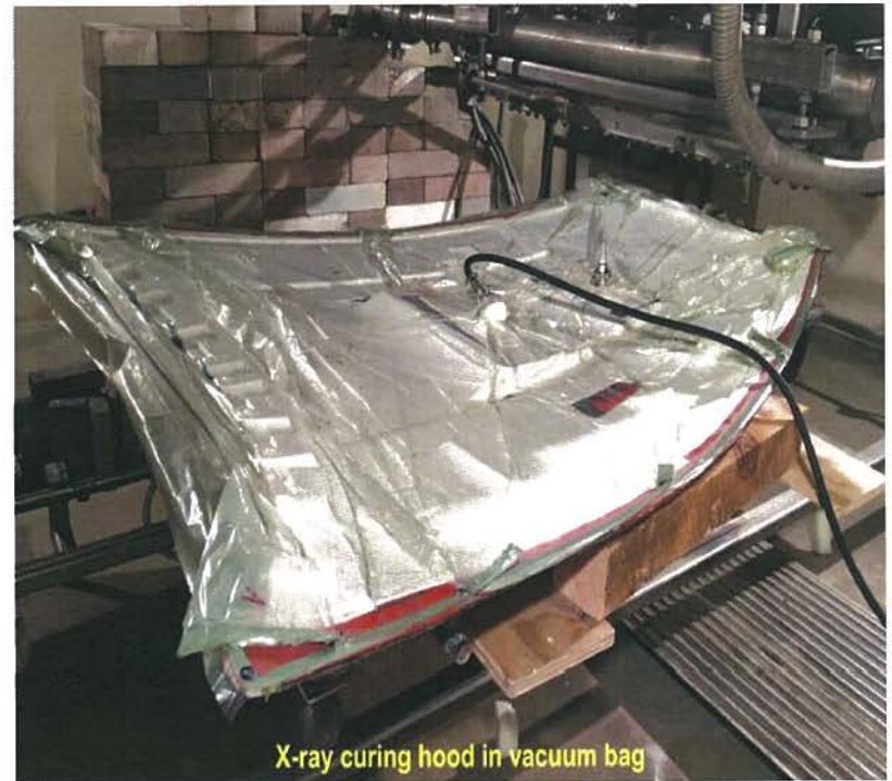
X-ray Curing a Hood in its Mold
