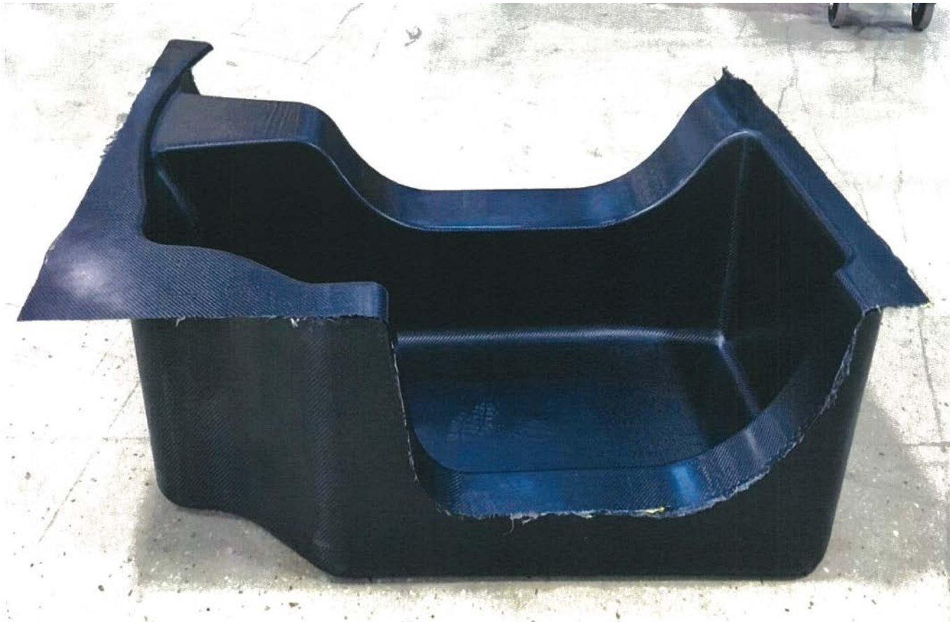
X-ray Cured Chassis (untrimmed)
